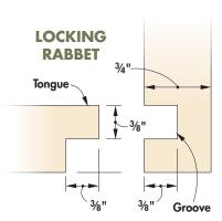
The interlocking parts of the tongue and dado form a sound mechanical joint and have a large glue surface for strength.
