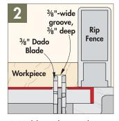
▲ Holding the workpiece firmly against the fence, cut the dado in a single pass.
