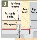
After attaching an auxiliary fence, rabbet the edge to form the mating tongue.
